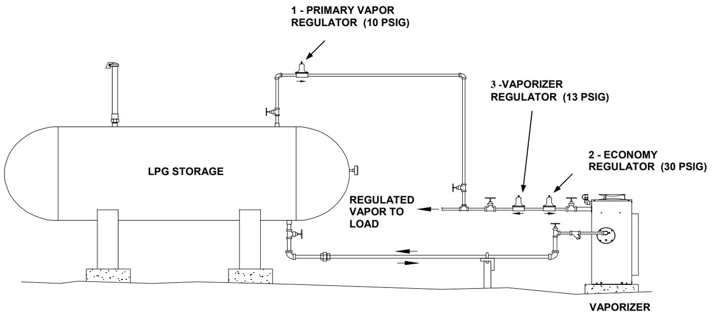
After installing the vaporizer, install and set the regulators from the economy kit as follows:
