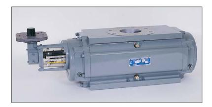
Dresser now offers a new version of the ROOTS® 23M rotary gas meter. Our 23M232 includes four inch flanged connections and a 232 PSIG (16 bar) maximum working pressure. This new design complements our standard six inch 23M175. With a maximum capacity of 385 MSCFH (10,895 Nm³ per hour) Dresser's new 23M is an ideal measurement solution for a wide array of applications.
