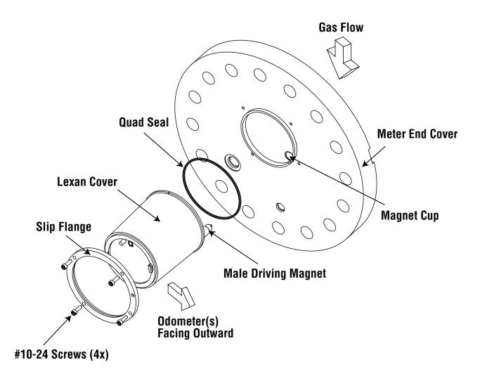
Figure 11- Assembling Series 3 Accessory to meter end cover.
