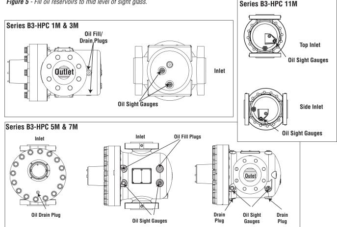
Figure 6 - Oil fill/drain plugs and oil level sight gauge locations.
