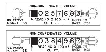
*Figure 8* - Non-Compensated Series 3 Imperial unit odometer for 1M (Top) and 7M (Bottom).
