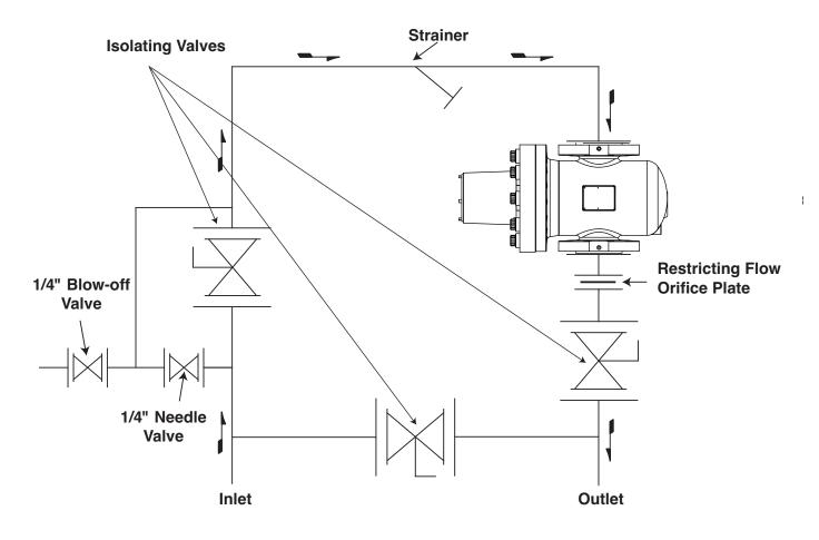
Figure 2 - Top Inlet Configuration for Series B3 Meter.
