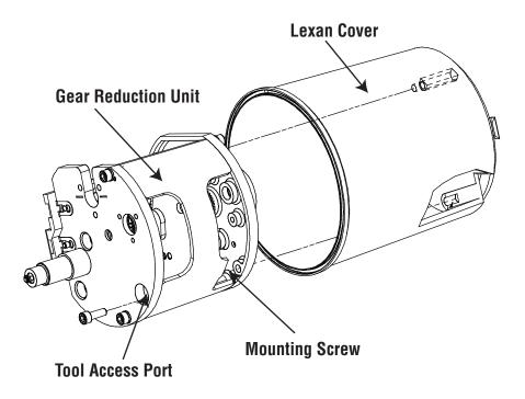
Figure 12 - Exploded view of Gear Reduction Assembly and Lexan® Cover.
