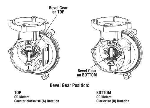
Figure 15 - Placement of bevel gears determines rotational direction.
