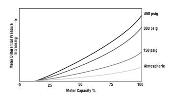
**Figure 17** - Differential Curves change as pressure increases.
