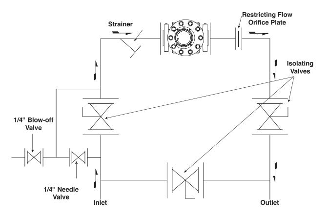
Figure 3 - Side Inlet Configuration for Series B3 Meter.
