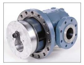
The bypass valve opens when meter differential reaches 6.5 psi (180 in.  $H_2O$ ), as tested with Natural Gas on the 1M and 3M, and 7.2 psi (200 in.  $H_2O$ ) for the 5M and 7M.
